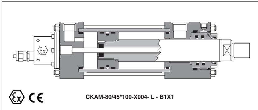
CKA cylinders are derived from standard CK (tab.B137) with certification according to ATEX 94/9/CE. They are designed to limit the external surface temperature, according to the certified class, to avoid the self-ignition of the explosive mixtures potentially present in the environment. CKAM servocylinders are equipped with ex-proof built-in digital magnetostrictive position transducer, ATEX certified.
