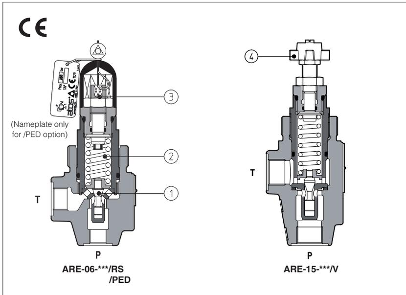
**ARE** are poppet type, directed operated pressure relief valves, with threaded ports for in line mounting.
