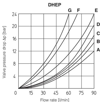
**9 OPERATING LIMITS** based on mineral oil ISO VG 46 at 50°C
