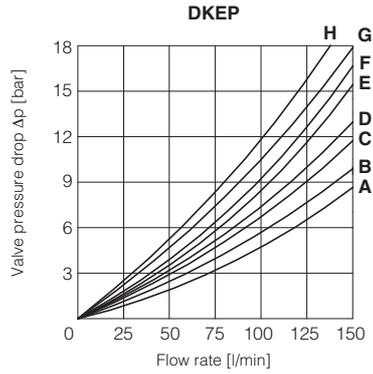
**13 OPERATING LIMITS** based on mineral oil ISO VG 46 at 50°C
