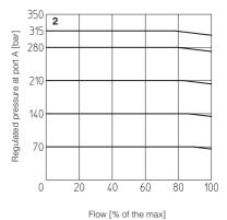
9.3 Pressure drop/flow diagrams with reference signal "null"
