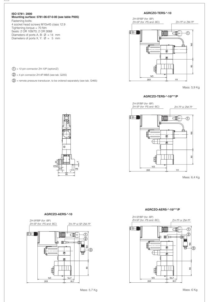
ISO 5781: 2000 Mounting surface: 5781-08-10-0-00 (see table P005) Fastening bolts: 4 socket head screws M10x45 class 12.9 Tightening torque = 70 Nm Seals: 2 OR 109/70 ; 2 OR 4100 Diameters of ports A, B:  $\emptyset$  = 22 mm Diameters of ports X, Y:  $\emptyset$  = 5 mm
