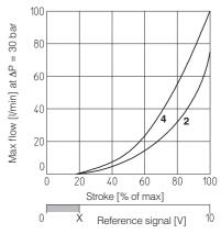
X = Threshold for bias activation depending to the valve type and amplifier type
