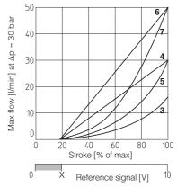
$\mathbf{X} = \text{Threshold}$  for bias activation depending to the valve type and amplifier type
