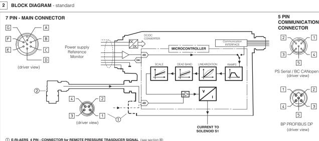
(2) E-RI-TERS CONNECTION for INTEGRAL PRESSURE TRASDUCER SIGNAL
